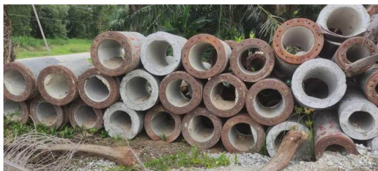
Cut-piles to be re-purposed as sinkers for the pontoon's mooring lines.
